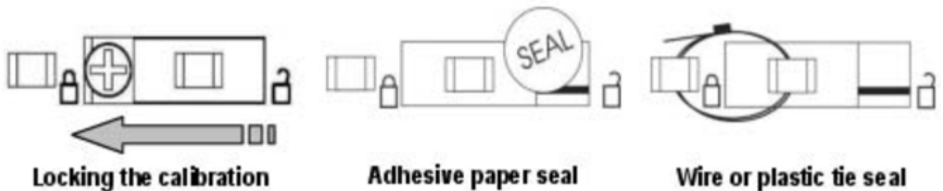
Figure 4-1. Locking and Sealing the Calibration Lock Switch.
