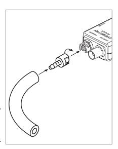
Note: Do not allow liquid to enter the pressure port.
