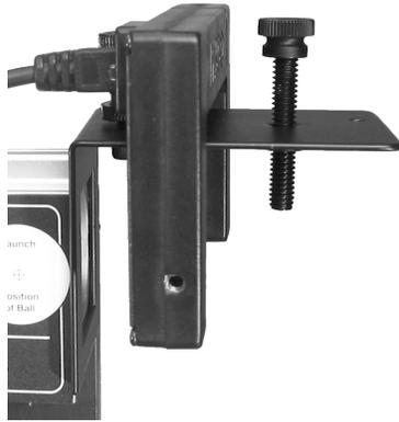
5. Connect a photogate as shown to measure the initial speed of the fired ball (optional). Since the photogate beam passes through the center of the ball's path, the velocity of the ball is calculated by the following equation:
