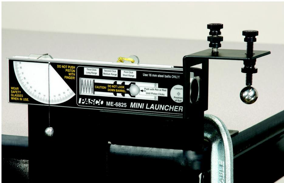
3. Slide the Drop Shoot Bracket into the groove on the bottom of the Projectile Launcher.
