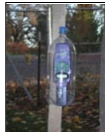
Figure 1: Weather Sensor and Xplorer suspended in plastic 2-liter bottle
