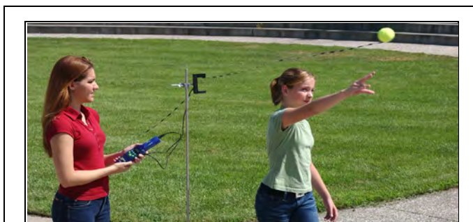
Figure 6: Recording the Velocity of a Thrown Tennis Ball with Photogate Tape
