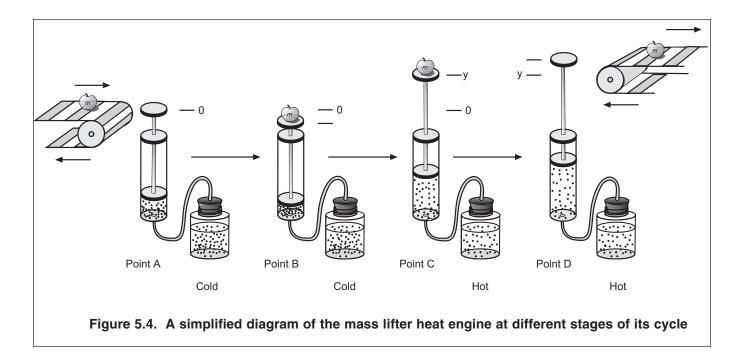
of a cycle carefully, indicating which of the transitions between points are approximately adiabatic and which are isobaric. You can observe changes in the volume of the gas directly and you can predict how the pressure exerted on the gas by its surroundings ought to change from point to point by using the definition of pressure as force per unit area.
