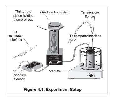
➤ Note: You can substitute a thermometer in the water container for the Temperature Sensor. Be sure to keep the tip of the thermometer from touching the bottom of the container.
