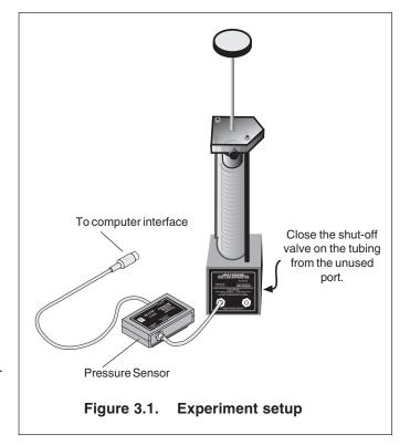
➤ Note: At pressures greater than 120 kPa, the relationship between pressure and volume may not be linear because of air leakage from the valves and ports at higher pressures.
