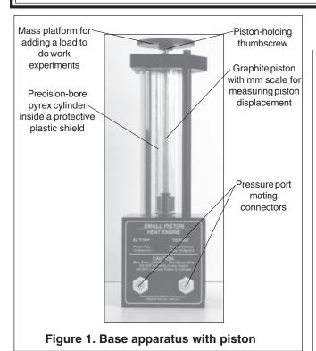
The Small Piston Heat Engine is designed with two pressure ports with quick-connect fittings for connecting to the air chamber tubing.
