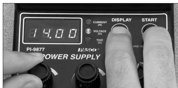
Setting “Hidden” Global Maximum voltage
