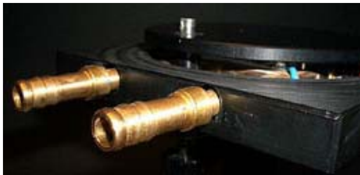
Fig. 7 Connection for cooling water circuit
