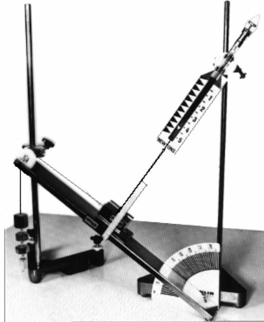
Simple set-up comprising 1 incline, 1 teaching dynamometer, 2 stands with rods, 2 fastening fixtures, 1 box of masses with hooks.
