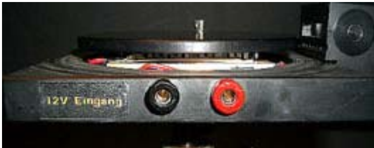
Fig. 5 Connections for supply voltage (12-15V / 8A)
